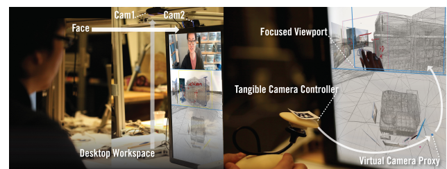
Figure 3. (a) AnnoScope system hardware configuration, (b)Tangible Camera Controller for navigation.
